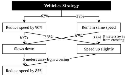
Fig. 3: Strategies of the vehicle in ambiguous situations with a reckless pedestrian simulated for crossing. (Based on [21].)
