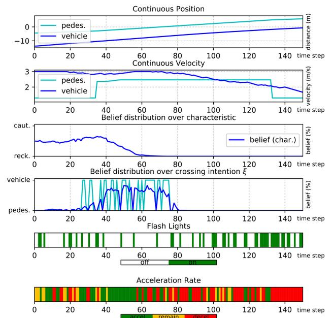
Fig. 7: A reckless pedestrian interacts with a vehicle equipped to flash its lights, communicating explicitly.
