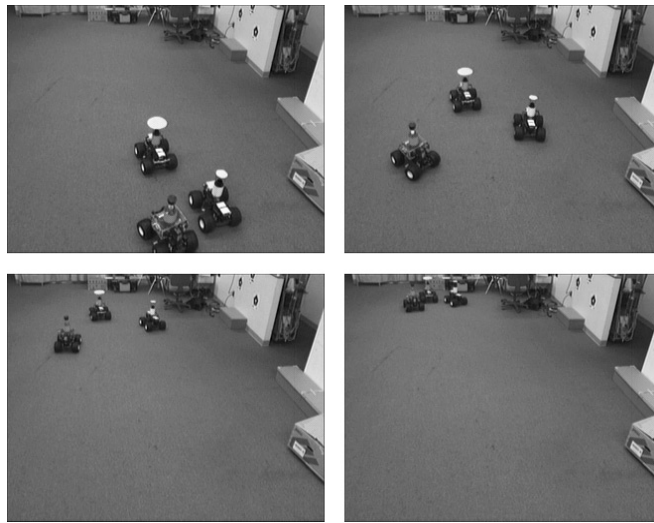
Fig. 14. Trajectory for two pursuer robots tracking a moving target robot in an obstacle-free environment.
